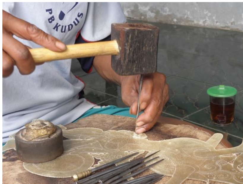
Figure 3-5. Proper chisel use for carving wayang kulit puppets
